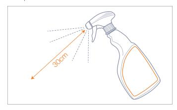
Spray clean surfaces and objects to be disinfected from a distance of 30cm so that they are completely moistened.
